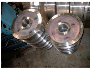
To realize the rough machining of the outer and inner contour surface of wheel blank, and clean up the spare parts of the blank quickly.
